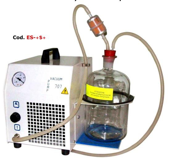
The Vacuum Pump ES-707 is used in biochemical, pharmaceutical and microbiological laboratories for emptying used in colourimetric and spectrometric analysis. It provides an easier filtration by Buckner funnels and provides sterilized solutions through special filter membrane.
